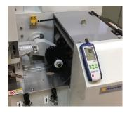
Water cooling system to prevent melting of products that are sensitive to heat.
