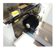
End seal support conveyor and adjustable end seal brush help to transition product seamlessly, along an even plane, to the belt fed out-feed conveyor.
