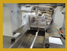
Delicate product conveyor with carrier card in-feed guide rails to handle product transitioning to the custom fixed former.
